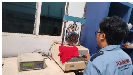
Gambar 8. Proses Pengujian Marshall
