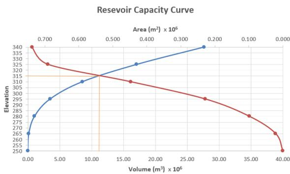
**Figure 3.7** Reservoir Capacity Curve
