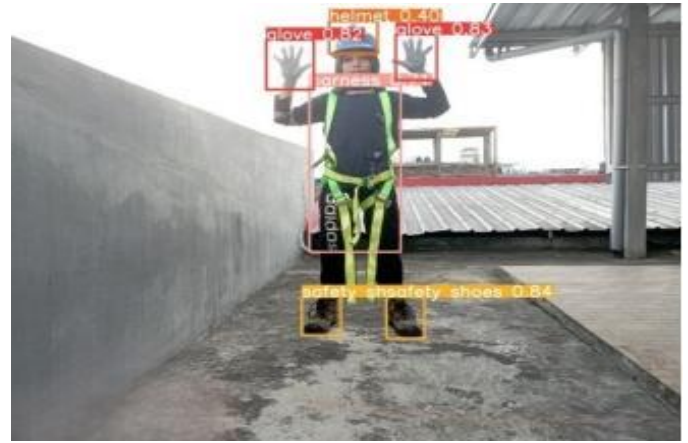
Figure 18. Result Of The 2nd Safety Equipment Detection Wearing Harness
