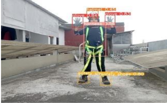
Figure 17. Result Of The 1st Safety Equipment Detection Wearing Harness
