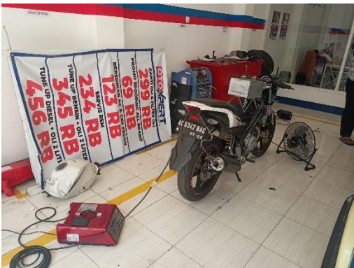
Gambar 2. Setting Peralatan Pengujian Emisi Gas Buang
