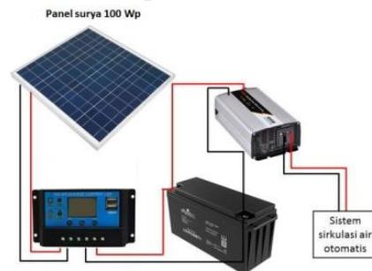
Gambar 17. Sistem Pompa Air Tenaga Surya
